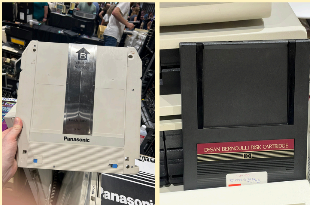
Two massive vintage data formats, WORM (Write Once Read Many) and Bernoulli (a kind of predecessor to the Zip Disk).
